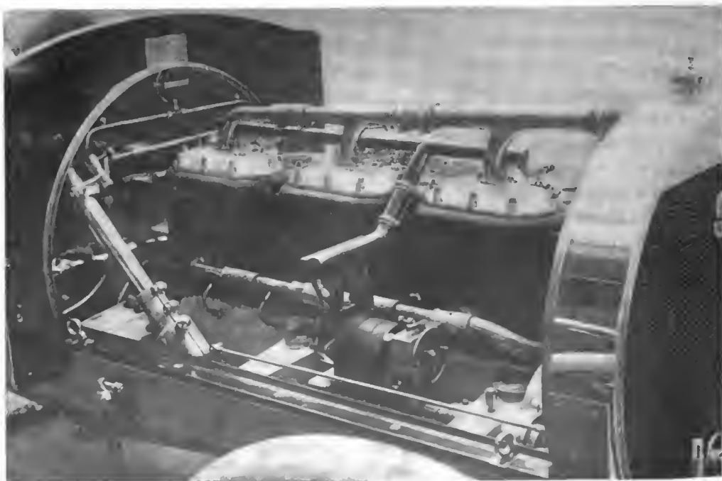
MAGNETO AND WATER INTAKE SIDE OF 45-HORSEPOWER SHEFFIELD SIMPLEX MOTOR.
